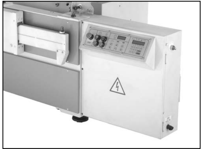
Figure 23. Control panel correctly set up.
